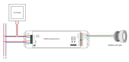
Note: When DALI address quantity is set as 1A and 4 PWM output channels are wired to LED loads simultaneously, please make sure the operation current of the LED loads does not exceed 1100mA.
