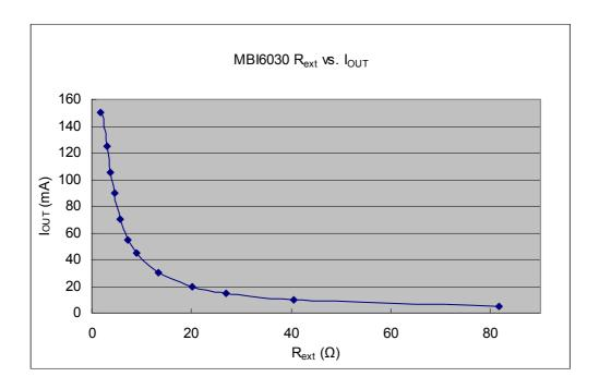
Also, the output current can be calculated by the equation:
