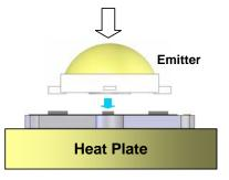
Put Emitter on MCPCB. Take the MCPCB out from Heat Plate within 10 seconds.
