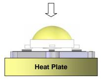
Put MCPCB on Heat Plate until Solder Paste melt. The Solder Paste sould be melted within 10 seconds. Take out MCPCB out from Heat Plate within 15 seconds.
