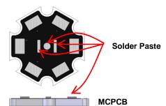
Use Solder Mask to print Solder Paste on MCPCB.
