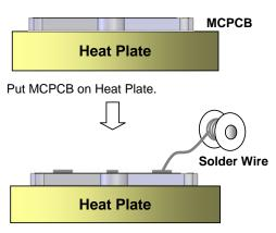
Place Solder Wire to the solder pad of MCPCB.
