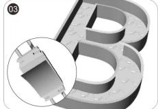
Peel off the release paper of double-sided adhesive tapes, then, stick modules on the installing surface for preliminary mounting
