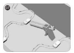
Adjust the modules to the best position, press the double-sided tape tightly and then fix by neutral glass glue.
