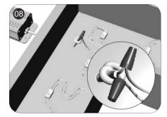
Please ensure that the "+" & "-" of the wires of modules are connected with those of power supply correctly.
