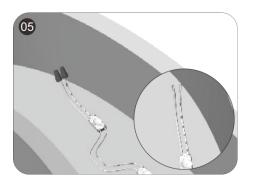
When the wires exposed in the last module, please peel off the insulation skin of wires about 10mm each, then, screw in terminals respectively, and dispose with waterproof, insulation protection
