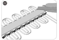
Cut the double-sided adhesive taps between every single unit by a cutter knife.
