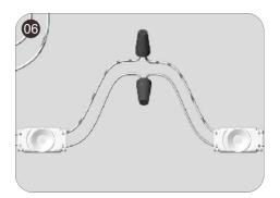
When connect the modules in series, peel off the insulation skin of wires of "+" and "-" about 10mm each, then, screw in terminals respectively, and dispose with waterproof, insulation, anti-corrosion protection and short-circuit prevention.
