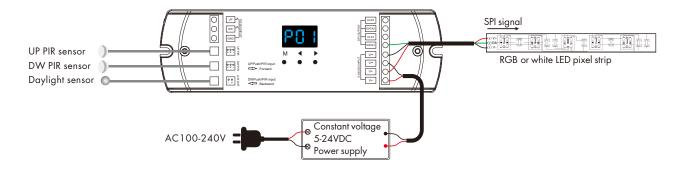
2. Stair light application, connect with PIR sensor, color or white light step control
