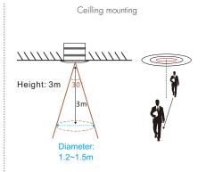
★ For wall mounting and ceiling mounting, note that the sensing holes are perpendicular to the direction of human movement.
