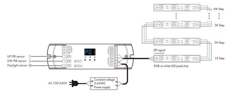
3. One push switch connect with multiple controllers for sequential switching control
