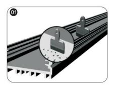
Make sure the mounting surface is clean before installation;
