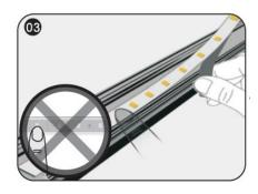
While sticking strips, peel off the release paper of the tape step by step. Don't peel off all release paper at a time to avoid getting your strip in a mess.
