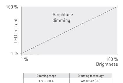
LC27MINI-DA-150-700 LED driver implements amplitude dimming technology across whole dimming range. Amplitude dimming offers the best available technology for dimming the light output in an accurate and flicker-free way to ensure high quality lighting in even the most demanding situations such as camera recording applications. Amplitude dimming technology complies with IEEE 1789-2015 recommendations of current modulation to mitigate health risks to viewers.
