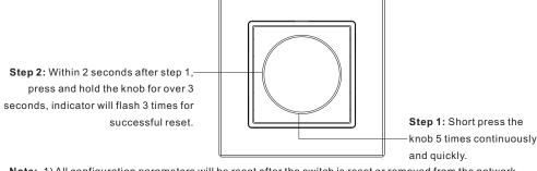
Note: 1) All configuration parameters will be reset after the switch is reset or removed from the network.
