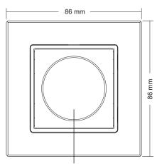
Click the rotary knob to switch ON/OFF paired Zigbee light devices
