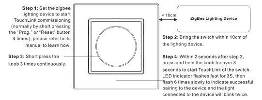
Note: 1) Directly TouchLink (both not added to a ZigBee network), please first factory reset both the switch (only need to reset when touchlink with 1st device) and device, each switch can link with max. 30 devices, please make sure the first linked device is always powered on when touchlink the switch with 2nd device and more devices.
