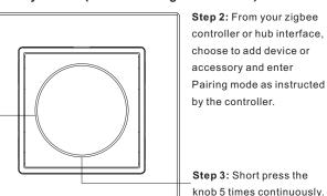
Note: 1) After pairing successfully, the switch information will appear on the controller or hub interface.
