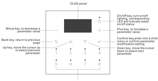
Scene keys 1-8, A. recall corresponding scene, corresponding LED will indicate Loads' on/off status. B. short press scene keys 1-8, DALI scenes 0-7 will be recalled in corresponding control area. B. double press scene keys 1-8, DALI scenes 8-15 will be recalled in corresponding control area. (Please refer to part 3.1.2 "scene saving" to learn how to save corresponding scene parameter.)
