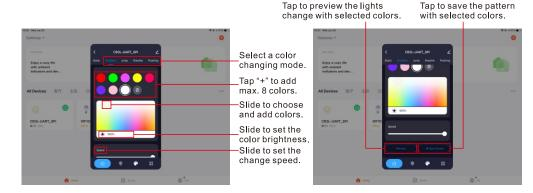
**Note:** 1) There are different styles of customize color patterns: Gradient, Jump, Breathe, Flashing, Rainbow and Stream, if a customized color pattern is saved as a scene, the user can recall it at the "Customize" column of "Preset Color Patterns".
