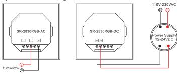
2)Receiver Connection Diagram for Multiple Units
